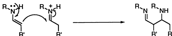
Figure 8. Possible reactions of imines in solution. The imine bond can hydrolyze in the presence of water to generate an amine and an aldehyde. The amine can be oxidized to an oxaziridine or a nitron. Or the double bond can tautomerize to form an enamine. A final possibility is tautomerization upon formation of the enamine, followed by nucleophilic attack on another imine, causing dimerization and polymerization.
